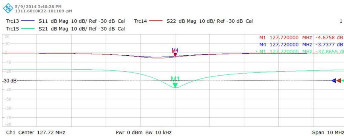
Figure 10: S-parameters measured on prototype body coil.
